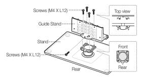
1. Connect the Guide Stand to the Stand using five screws (M4 X L12) as shown.
